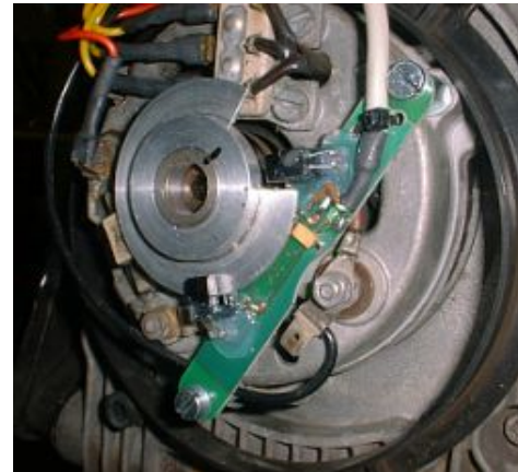
Installed pickup and sector disk
