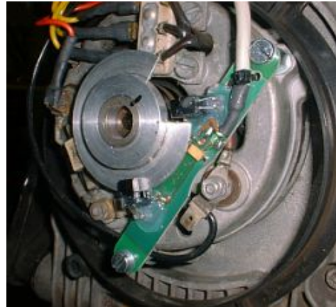
Figure 5 Installed pickup and sector disk
