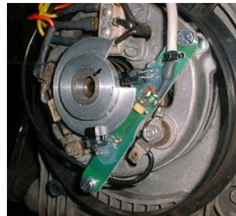
Installed pickup and sector disk
