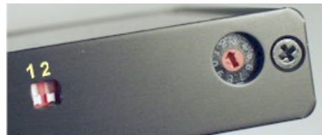
Figure 3 DIP switches and rotary switch.
