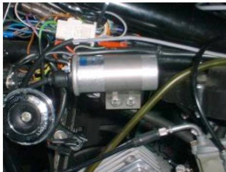
Figure 2 Mounting suggestion with PVL220 ignition coils.
