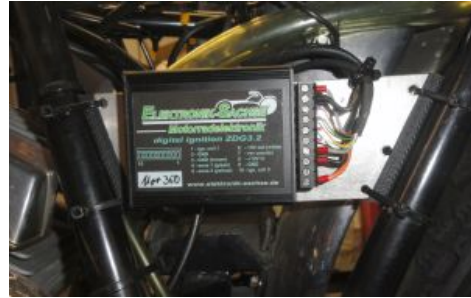
Figure 2.b The ignition box is mounted in the frame on a piece of sheet metal.
