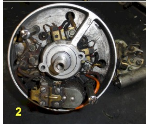
Figure 2.b Remove the components of the old ignition.
