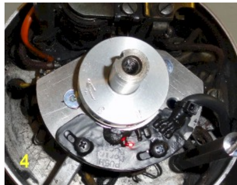
Figure 2.e Mount the magnet disk on the shaft.
