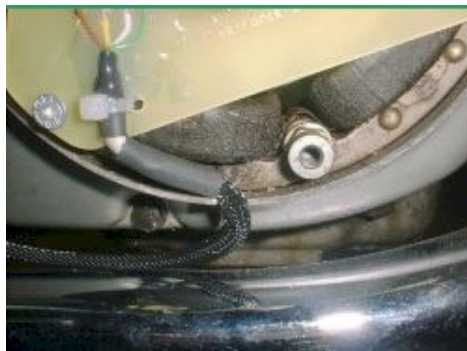
Figure 2 Routing the pickup lead through the cutout.
