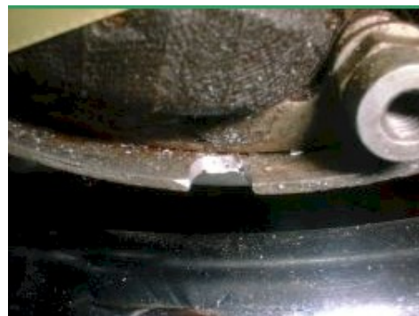
Figure 2 Cutout for the pickup lead.
