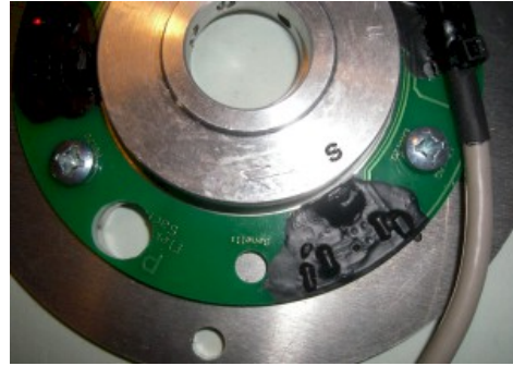
Figure 8.b The LED goes off when the piston is on TDC.
