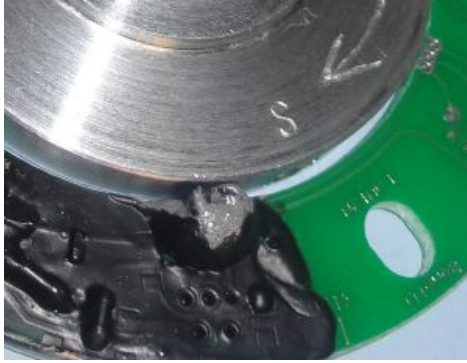
Figure 8.a The LED goes off with the N-magnet passing the sensor.
