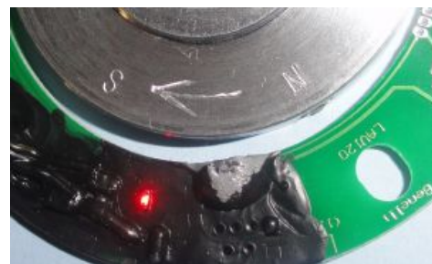
Figure 8.b The LED goes on with the S-magnet passing the sensor.
