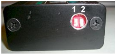
Figure 4 DIP switches and advance curve selection.
