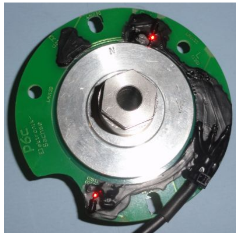
Figure 6 Pickup with driver sleeve and magnet disk.
