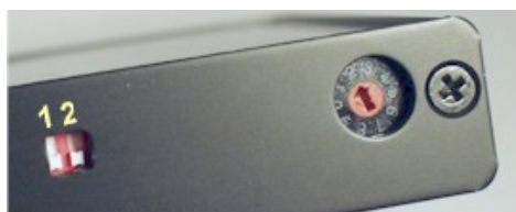
Figure 3 DIP switches and rotary switch.
