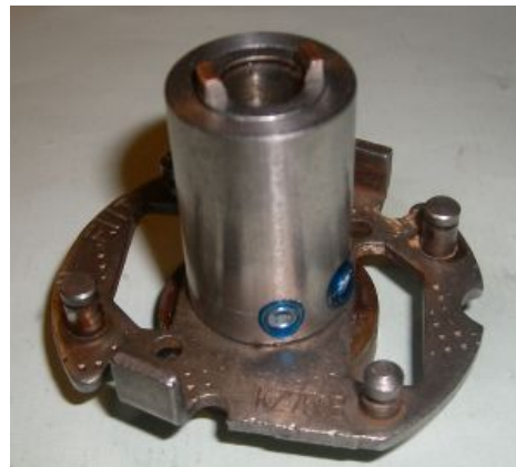
Figure 2 Driver sleeve mounted on the original shaft.
