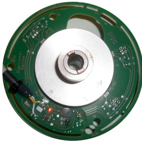
Figure 7 Pickup with driver sleeve and magnet disk.
