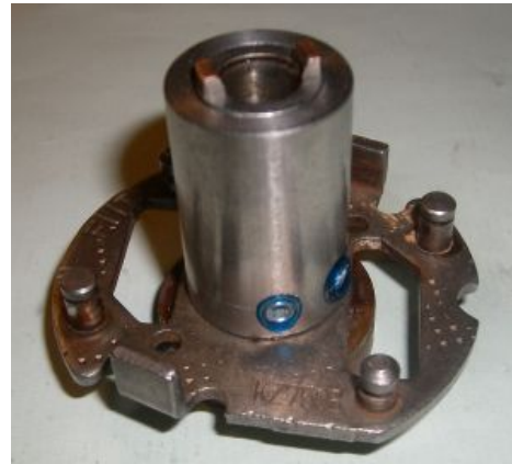
Figure 2 Driver sleeve mounted on the original shaft.
