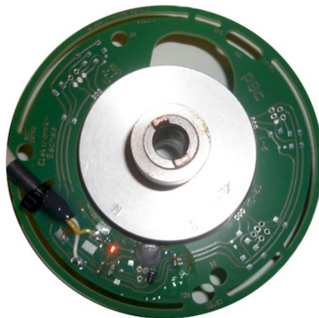
Figure 7 Pickup with driver sleeve and magnet disk.
