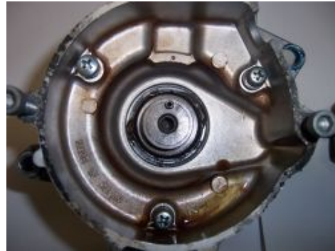
Figure 2.b Driver sleeve mounted on the shaft.
