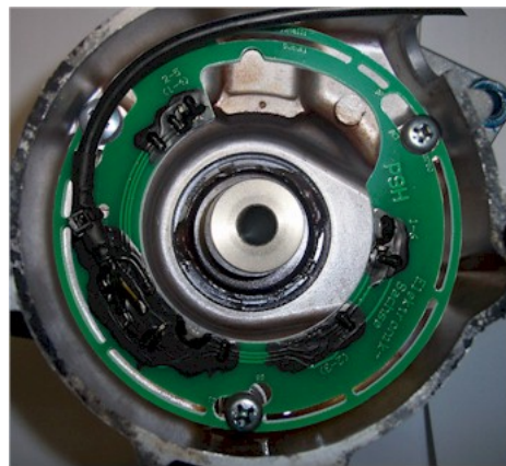
Figure 2.d Mounted pickup and driver sleeve. The magnet disk is not mounted, yet.
