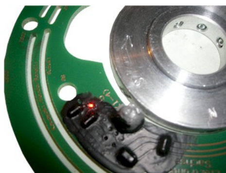
Figure 6.b The LED goes on when the S-magnet passes the sensor and off when the N-magnet passes the sensor.
