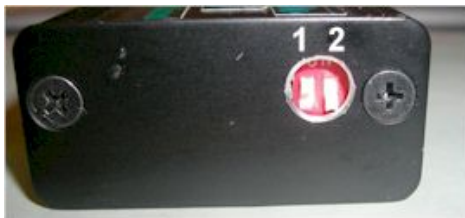
Figure 3 DIP switches and advance curve selection.
