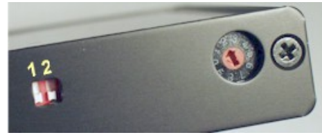
Figure 6 DIP switches and rotary switch.
