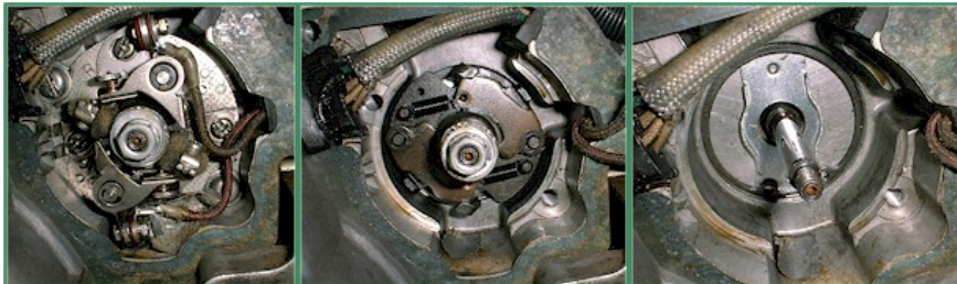
Figure 1 Remove the original contact breaker plate and the advance unit
