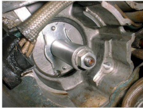
Next push the driver onto the shaft and fasten it with the nut.
