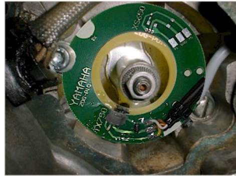
Then fasten the printed circuit board with the provided M6 screws.
