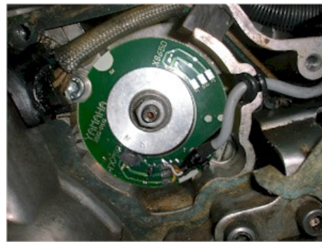
At last put the magnet disk onto the sleeve hub, but do not tighten the set screws yet.
