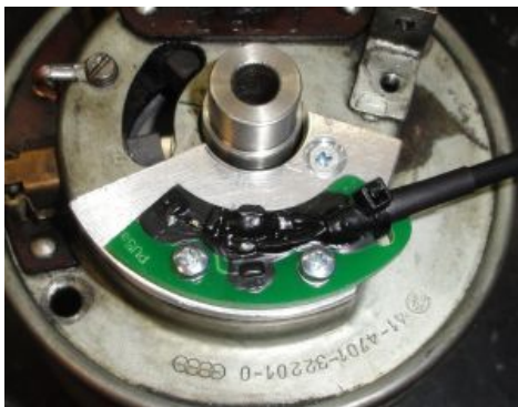
Fit the sensor plate with the two provided M3 screws.
