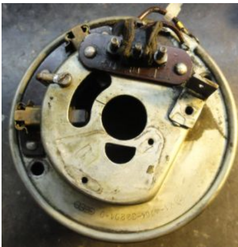
Remove the contact breaker plate and the advancer, the felt slider too.
