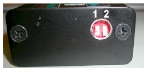
Figure 4 DIP switches and advance curve selection.
