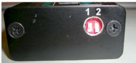
Figure 4 DIP switches and advance curve selection.
