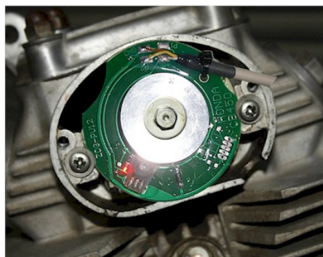
Fitting of the sensor plate (photomontage)
