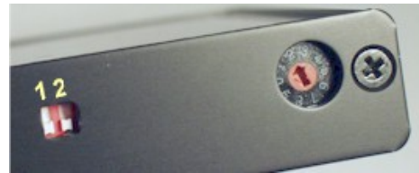
Figure 4 DIP switches and rotary switch.
