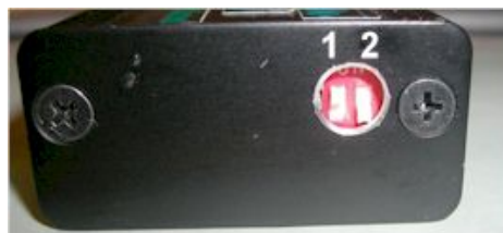
Figure 3 DIP switches and advance curve selection.
