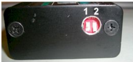
Figure 4 DIP switches and advance curve selection.
