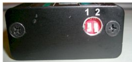
Figure 4 DIP switches and advance curve selection.
