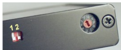
Figure 3 DIP switches and rotary switch.
