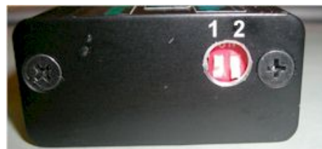
Figure 3 DIP switches and advance curve selection.
