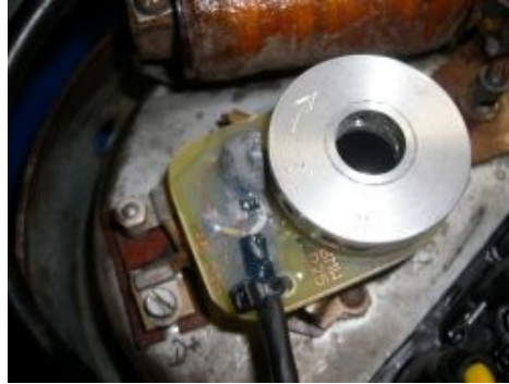
Unscrew the centre screw and tighten it again with the driver sleeve. At last push the disk onto the sleeve but don't tighten the set screws.
