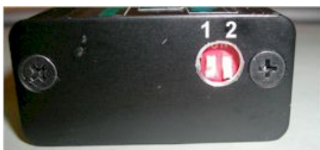
Figure 4 DIP switches and advance curve selection.
