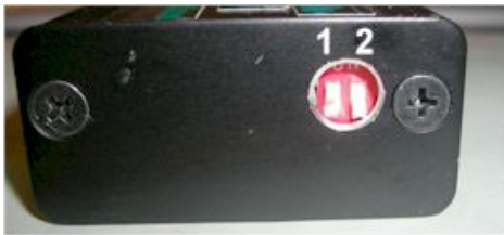
Figure 3 DIP switches and advance curve selection.
