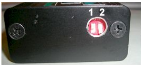
Figure 4 DIP switches and advance curve selection.
