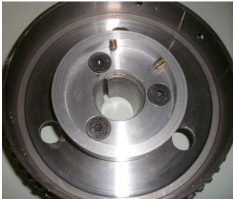
Mounting the magnet disk in the original flywheel.
