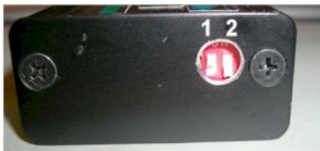
Figure 4 DIP switches and advance curve selection.
