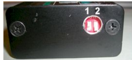
Figure 3 DIP switches and advance curve selection.
