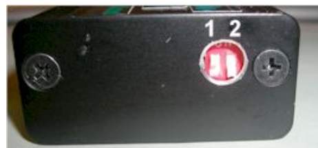
Figure 3 DIP switches and advance curve selection.
