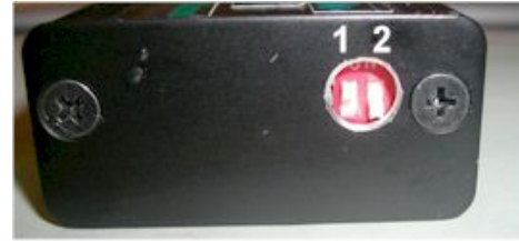
Figure 3 DIP switches and advance curve selection.
