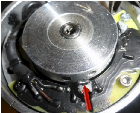
Figure 3 Ensure correct alignment of magnet disk and sensor.
