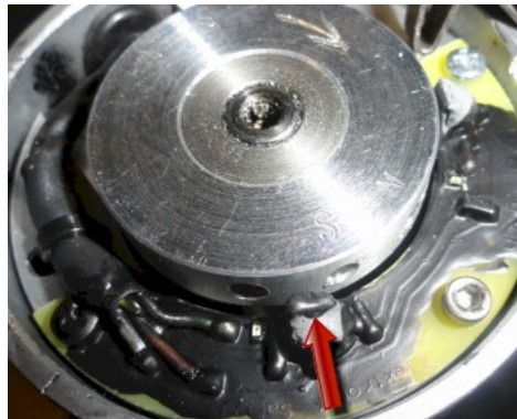
Figure 2 Ensure correct alignment of magnet disk and sensor.
