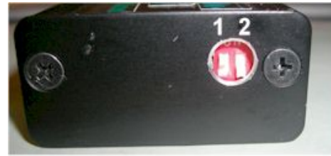
Figure 3 DIP switches and advance curve selection.
