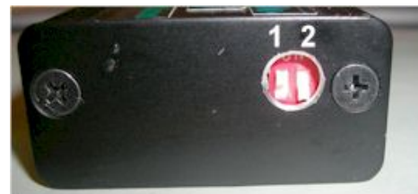
Figure 4 DIP switches and advance curve selection.
