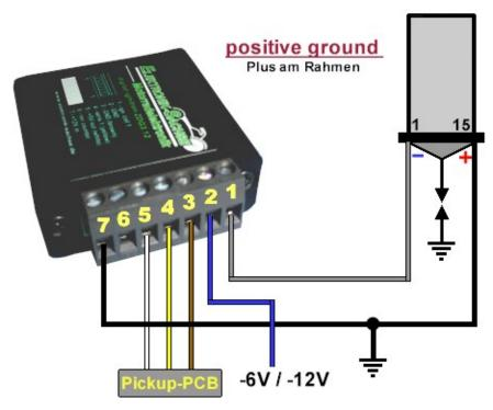
Positive ground – Plus connected to frame
