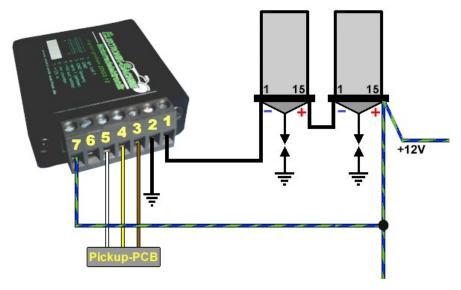
Negative ground – Minus connected to frame, two 6 V coils connected in series.
