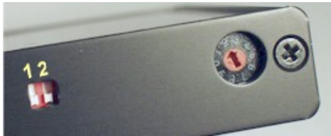
Figure 4 DIP switches and rotary switch.
