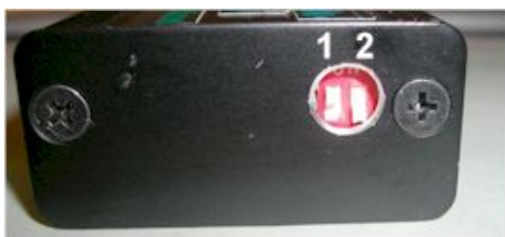
Figure 4 DIP switches and advance curve selection.
