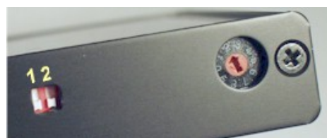
Figure 7 DIP switches and rotary switch.
