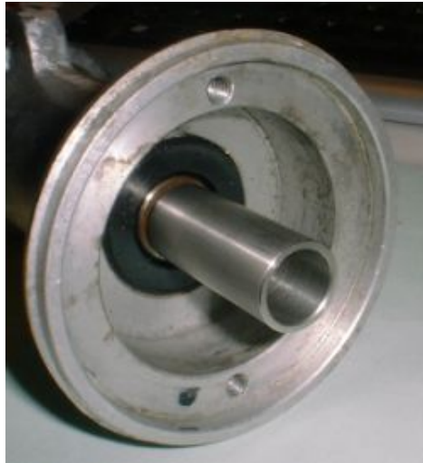
Figure 2 Remove the original ignition components and mount the driver sleeve.
