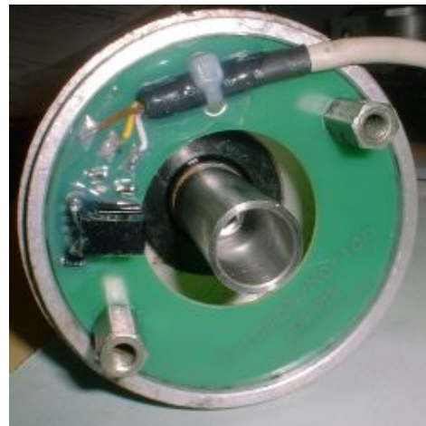
Figure 2.b Mount the pickup (older version is shown here).
