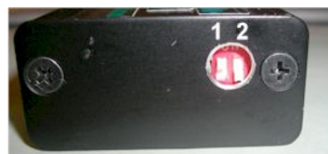
Figure 4 DIP switches and advance curve selection.
