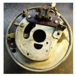
Remove the contact breaker plate and the advancer, the felt slider too.
