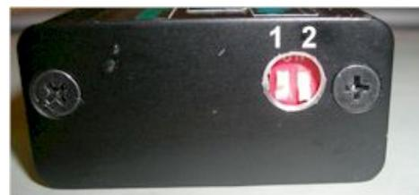
**Figure 4** DIP switches and advance curve selection.
