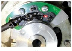
Finally secure the set screws with medium strength thread lock compound. This is best done after the initial setup is finished and accurate. Then remove only one of the set screws, so the position of the magnet disk doesn't change. Apply a small amount of thread lock compound and re-tighten the set screw. Repeat with the other set screw(s).
