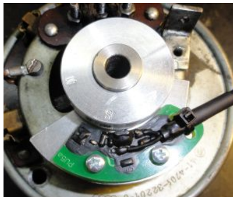
Last, push the magnet disk onto the sleeve (rotation direction right), but do not tighten the set screws in the disk.
