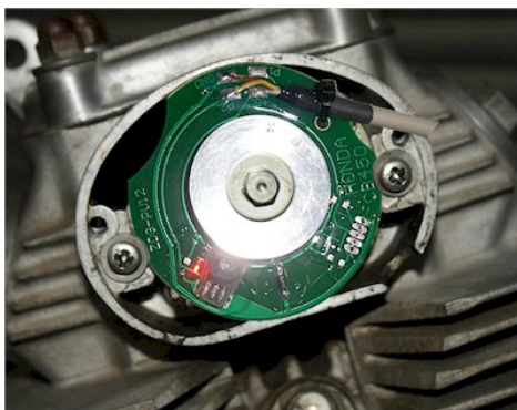
Fitting of the sensor plate (photomontage)
