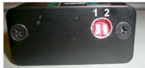
Figure 4 DIP switches and advance curve selection.
