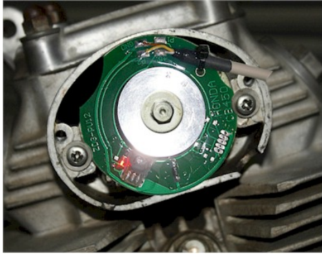
Fitting of the sensor plate (photomontage)
