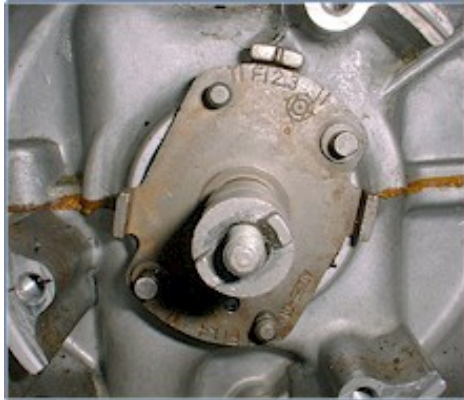
Figure 2 Using the original sleeve with our magnet disk. This is the recommended method if this kit includes no driver sleeve.
