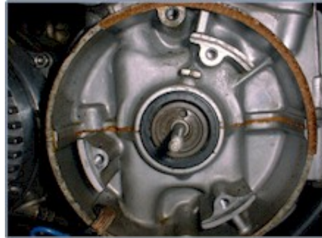
Figure 2 Removal of the original sleeve so that our driver sleeve can be mounted.
