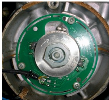
Figure 3 Completed fitting of our magnet disk and driver sleeve.
