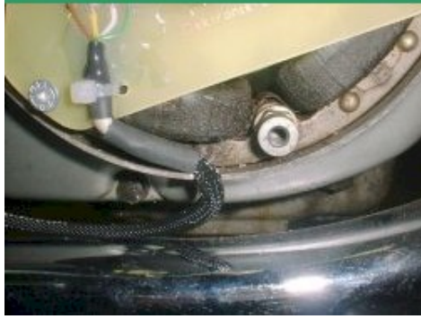
Figure 2 Routing the pickup lead through the cutout.
