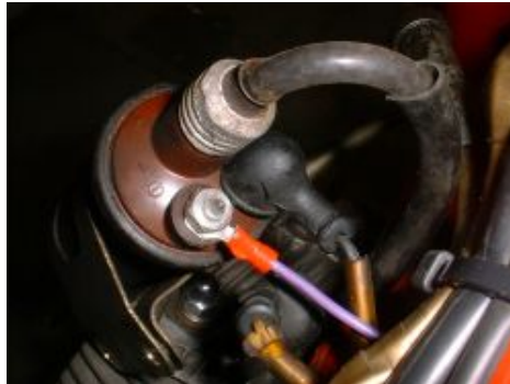
Figure 3 Mounting suggestion of the left ignition coil.
