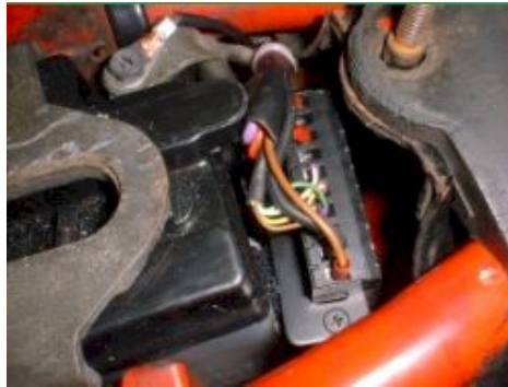
Figure 2 Ignition box mounting suggestion.
