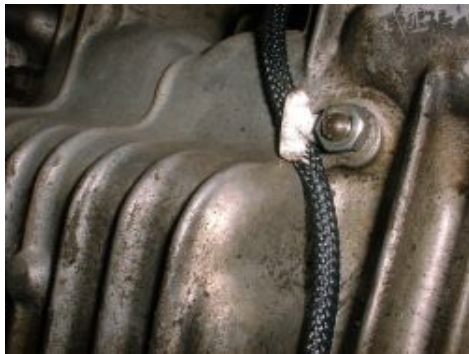
Figure 2 Pickup lead protection.
