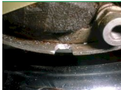
Figure 2 Cutout for the pickup lead.
