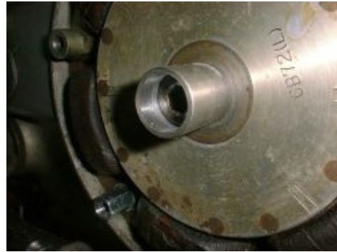
Figure 2 Mounting the driver sleeve.
