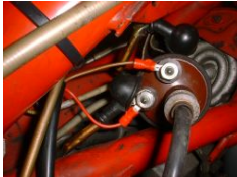
Figure 3 Mounting suggestion of the right ignition coil.
