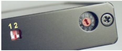
Figure 10 DIP switches and rotary switch.
