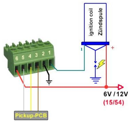
Figure 2 Circuit diagram.
