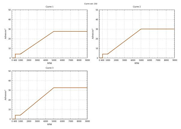
Figure 7 Selectable ignition curves.
