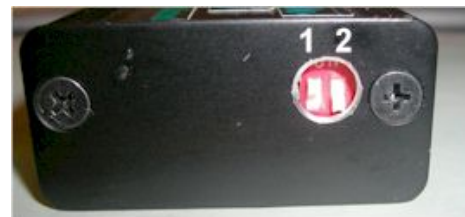
Figure 4 DIP switches and advance curve selection.
