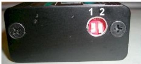
Figure 4 DIP switches and advance curve selection.
