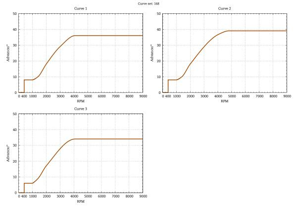
Figure 5 Selectable ignition curves.
