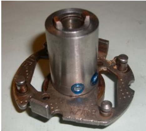
Figure 2 Driver sleeve mounted on the original shaft.
