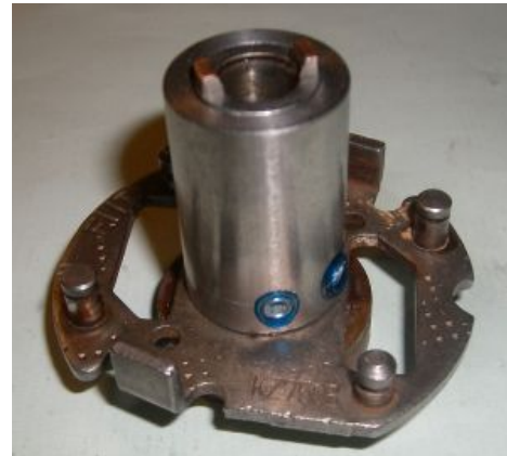
Figure 2 Driver sleeve mounted on the original shaft.
