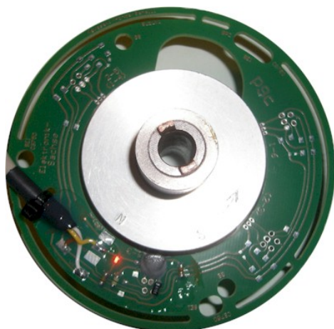
Figure 7 Pickup with driver sleeve and magnet disk.
