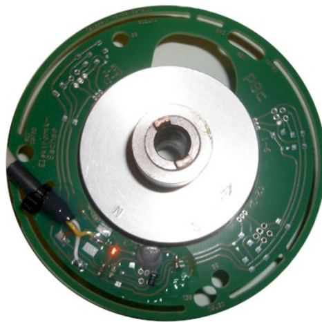
Figure 7 Pickup with driver sleeve and magnet disk.
