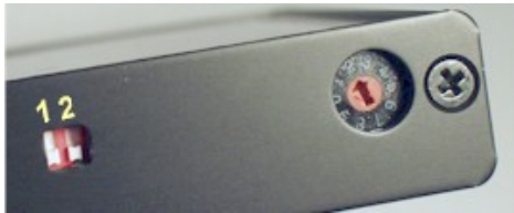
Figure 8 DIP switches and rotary switch.
